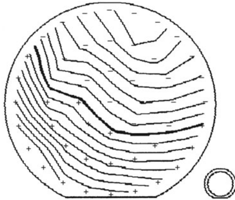
Fig. 2.3. Wafer polished for 60 seconds on Strasbaugh 6DS with no carrier rotation. Pre-polish wafer thickness was 10,000 \text{ \AA} and the dark line is the post-polish 7500 \text{ \AA} contour line. The contour line spacing is 250 \text{ \AA} . The leading edge is at the top of the wafer. Courtesy of David Evans, private communication
